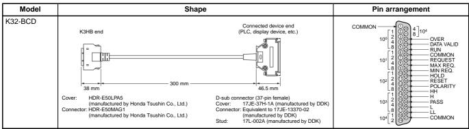
Note: The BCD Output Cable has a D-sub plug. Cover: 17JE-37H-1A (manufactured by DDK); Connector: equivalent to 17JE-23370-02 (D1) (manufactured by DDK)
