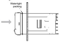
Insert the adapter into the grooves on the left and right sides of the rear case and push until it reaches the panel and is fixed in place.
